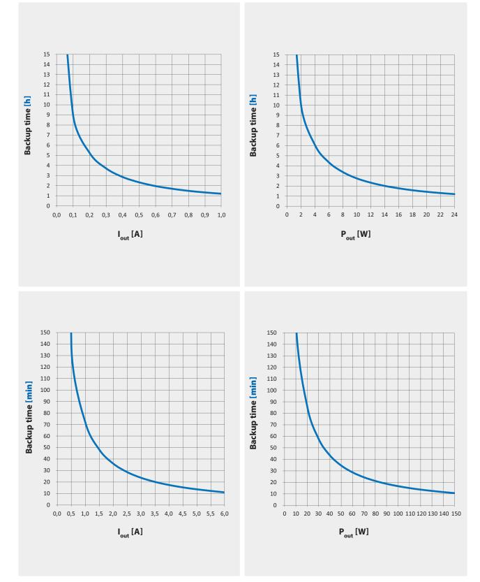
\*Backup time depends on battery capacitance, load and temperature. At very high or low temperatures a reduction of backup time occurs. Unless otherwise specified, the values apply to measurements at +25 °C
